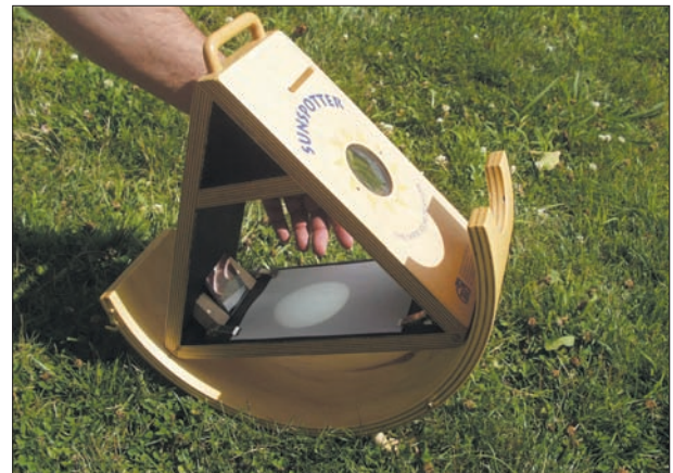
A small sunspot telescope, with the beam folded by reflection of several mirrors to make the system compact and easy to set up.
